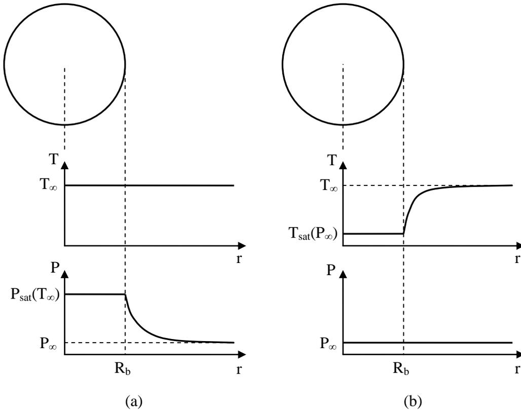
Figure 1. Pressure and temperature fields in and around vapor bubbles for (a) inertia dominated growth and (b) thermal diffusion dominated growth.
