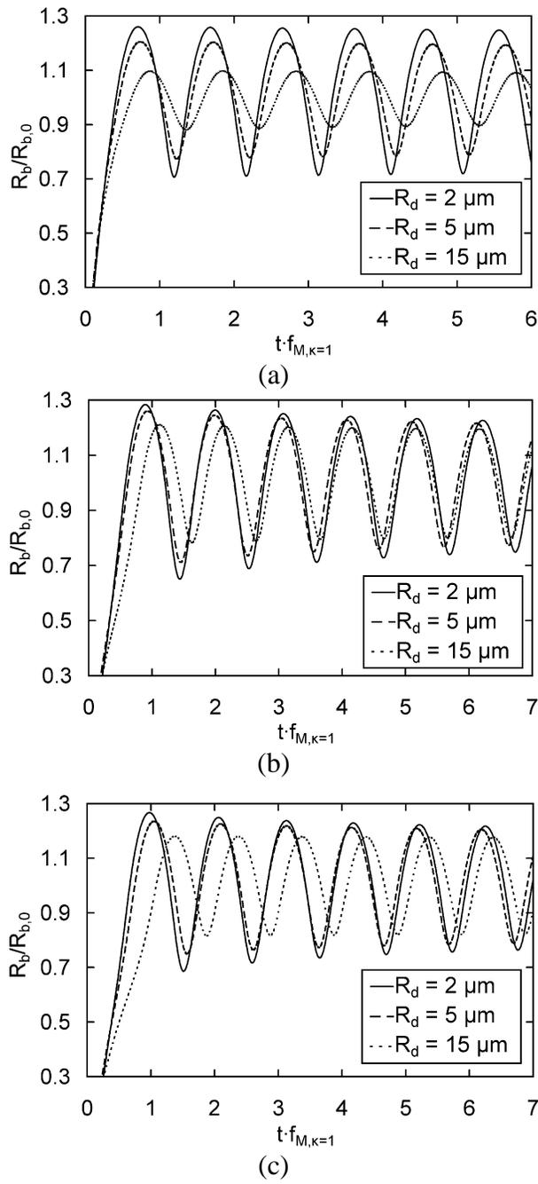
Figure 6. Oscillation of (a) water vapor bubble in mineral oil,  $\Delta T = 40 \text{ }^\circ\text{C}$ , (b) pentane vapor bubble in water,  $\Delta T = 20 \text{ }^\circ\text{C}$ , and (c) FC-72 vapor bubble in water,  $\Delta T = 20 \text{ }^\circ\text{C}$ .
